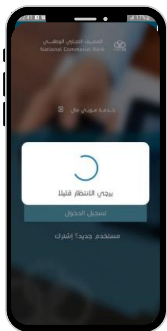
Fig. 1: Lack of system status feedback during a long-running operation.
